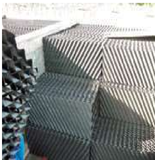
F-14.1.5-B-PVC media support made up of plastic
